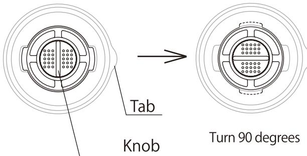
Turn the removable bottle spout so that the tab of the rim is pointing to the right. Set the filter inside the spout so that the knob is vertical. Twist the knob 90 degrees and confirm that the filter is securely set.
