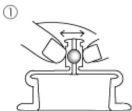
2. If water doesn't drip even if you have done the above, insert a stick with a round end, such as a chopstick, into the hole of the rubber valve and push the metal ball in order to remove it from the rubber valve.
